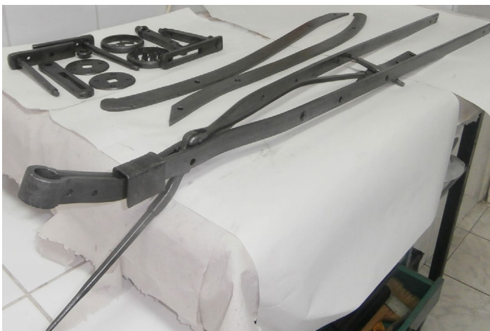
Sheet XI: Parts of Velocipede after metal cleaning Foto: Claudia Moței
